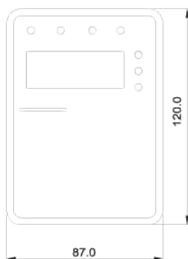
Figure A-11 Dimension of big keypad
