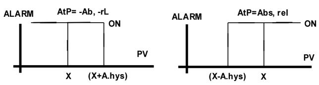
If Alarm mode (AtP) is selected as "SnS"; in case of sensor failure, measurement out of range or hardware fails (when "or" is displayed), OUT output is first OFF for TOf and then ON for Ton periodically. For continuous OFF, enter TOn=0 & TOf=0. For continuous ON, enter TOn=1 & TOf=0.
