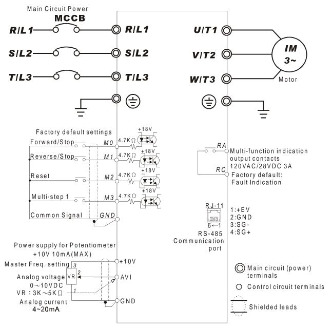
NOTE: Do not plug in a Modem or telephone line to the RS-485 communication port, permanent damage may result. Terminals 1 & 2 are the power source for the optional copy keypad and should not be used while using RS-485 communication.
