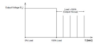
Additionally, if the IO is <150% but >100% for a prolong period of time (depending on the load), the Over Temperature Protection (OTP) will be activated due to high temperature on critical components. The power supply will then go into "Hiccup mode" until the fault is removed.
