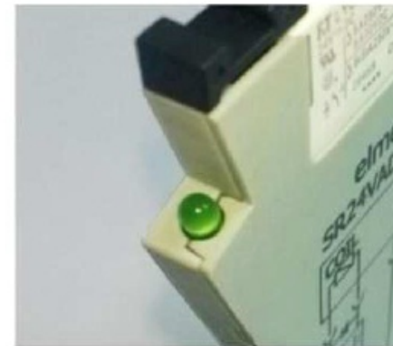
Relay Coil Energised Indication
