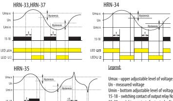
Umin - bottom adjustable level of voltage 15-18 - switching contact of output relay No.1 25-28 - switching contact of output relay No. 2
