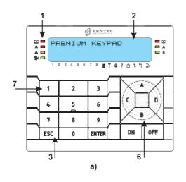
zer will start sounding a series of beeps in such manner that the operator could hear the sound level in real time. 2a) To increase the volume, press key **A** for a number of times and/or keep it pressed until the desired level is obtained: 2b) To lower the volume, press più volte and/or keep pressed key **B** until the desired level is obtained.
