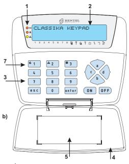
Figure 1 - a) PREMIUM LCD Keypad, b)CLASSIKA LCD Keypad.
