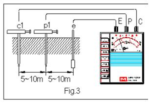
Where it is not possible to drive the auxiliary earth bars into a hard surface such as concrete ground, lay the earth bars there, covet them with a cloth and put water (preferably salt water). This may allow earth resistance measurements.
