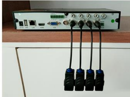
Baluns click together for a neat installation
