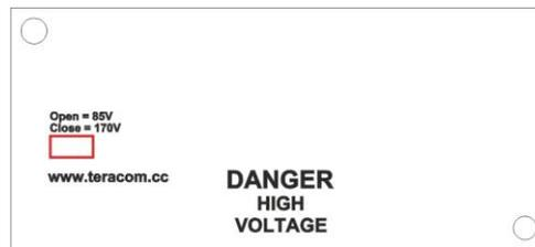
If the jumper is open detection level is 85VAC, if it is close, detection level is 170VAC.
