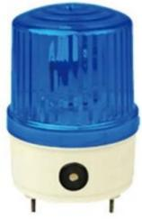
High brightness LED light tube light source life of 50,000 hours, saving energy, low heat, no maintenance; Steady / LED rotating, flashing functions Optional; flash frequency 90-150 beats / min; Material: shade -AS, base -ABS; protection class IP45; products with buzzer volume: 85dB above; installation way: bolt-
