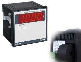
Designed for industries that do not have much spare places in there current transformers or to reduce the costs. It contains a small current transformer. It measures the current in the cable that will be passed through a hole in the current transformer.
